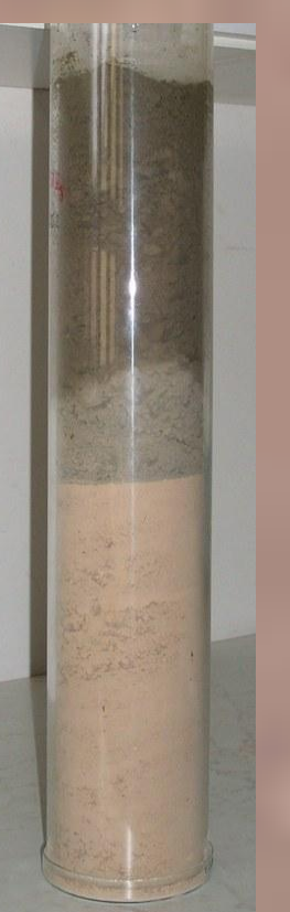
Figure 5: Water infiltration into the top (grey soil) layer (25 cm) after 5 days. Bottom layer: 25 cm brick.
