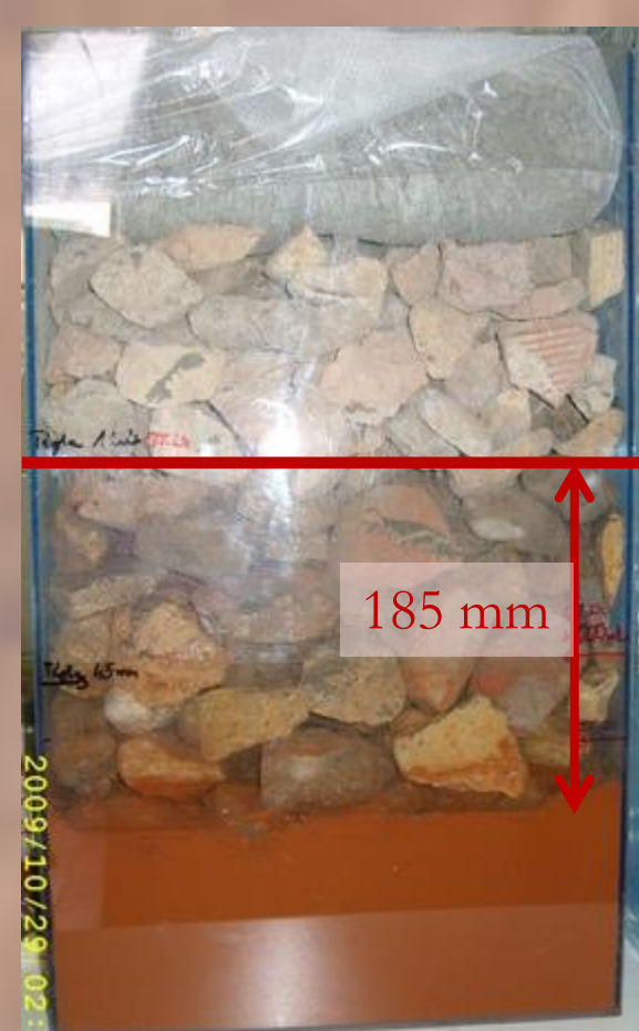
Figure 3: Water suction from red mud + 45 mm precipitation by coarse brick (30–50 mm) after 1 week
