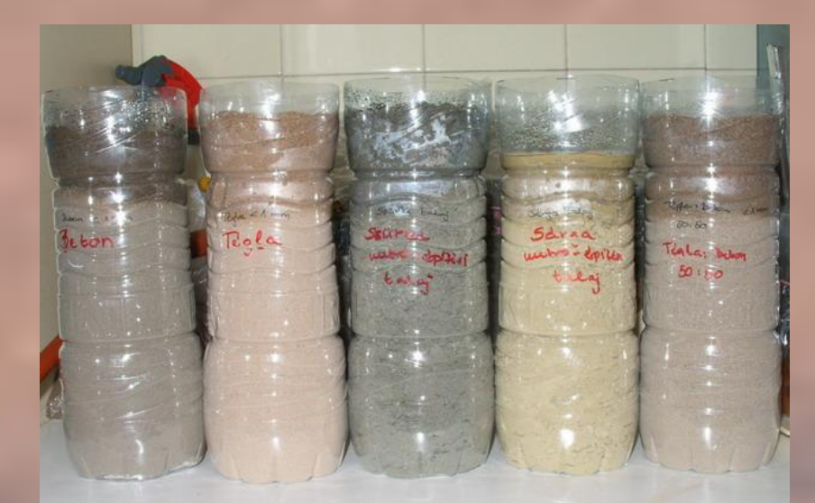
Figure 4: Wastes in PET bottles: measurement of infiltration
