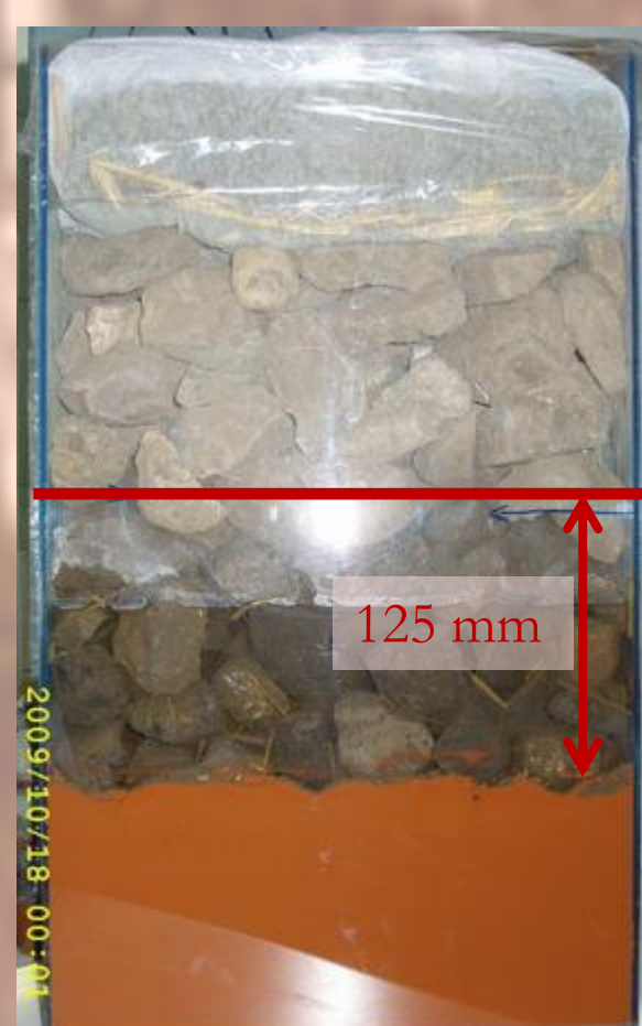
Figure 2: Water suction from red mud + 45 mm precipitation by coarse concrete (30–50 mm) after 1 week
