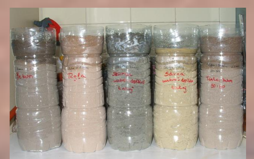
Figure 4: Wastes in PET bottles: measurement of infiltration
