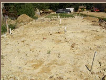
Fig. 10. The untreated plot: plants were not able to grow due to high acidity and toxic metal concentrations
